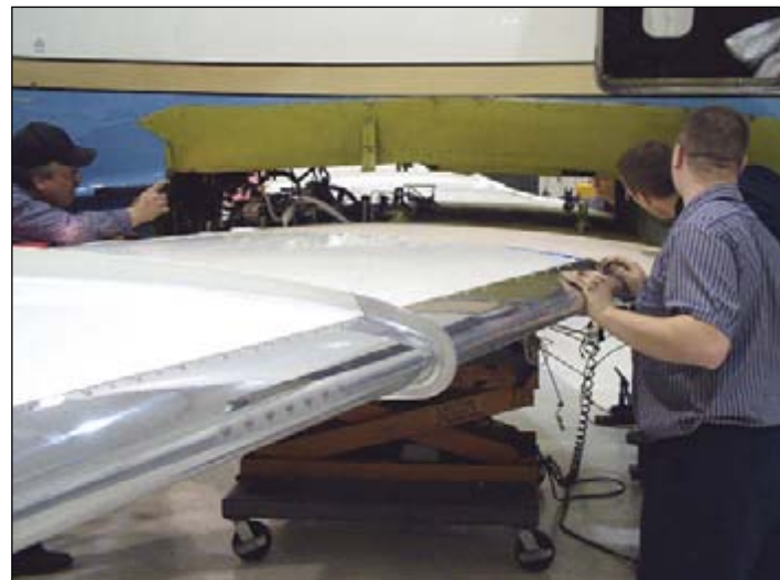
The Battle Creek team has seen many Learjets in for service since the new authorization. One memorable job was a fuel leak repair on a Lear 60 that required the removal of the wing. The leak was found and repaired quickly, and the customer was happy with his experience with the new team.
