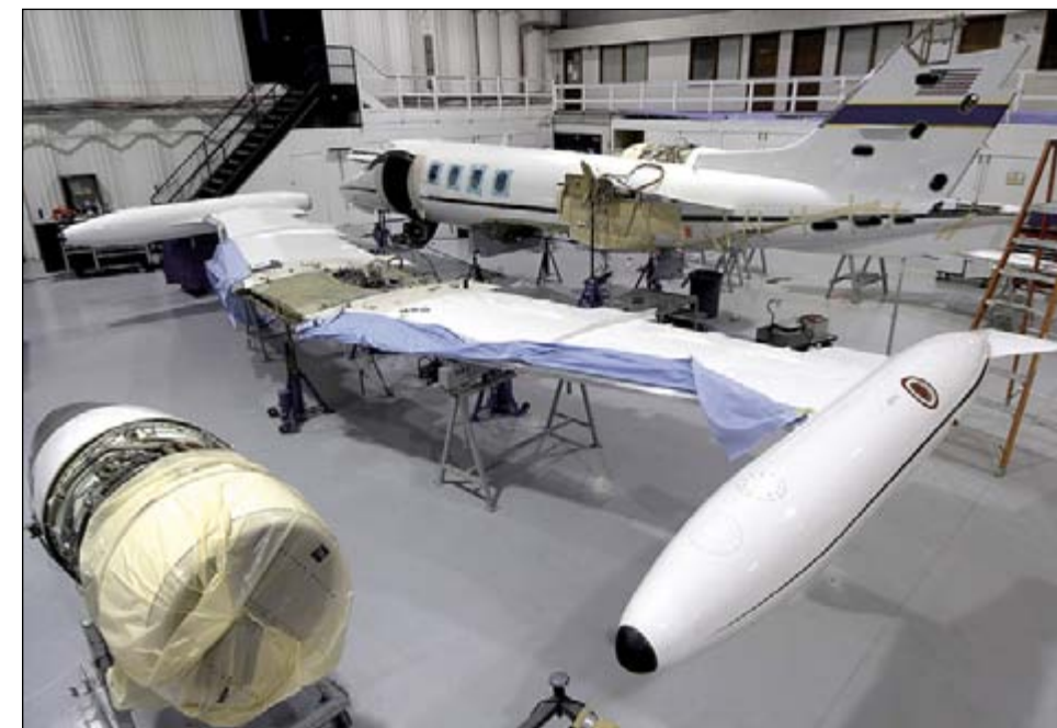
The Battle Creek team has seen many Learjets in for service since the new authorization. One memorable job was a fuel leak repair on a Lear 60 that required the removal of the wing. The leak was found and repaired quickly, and the customer was happy with his experience with the new team.
