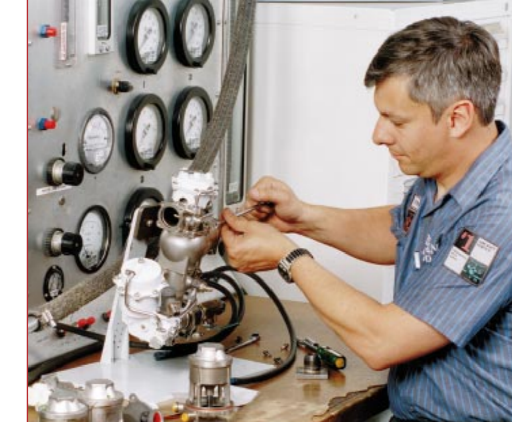
Accessory Technician III Rich Kasl prepares to test a bleed switching valve. Duncan Aviation can now repair and overhaul components associated with the AlliedSignal TFE731 engine.
