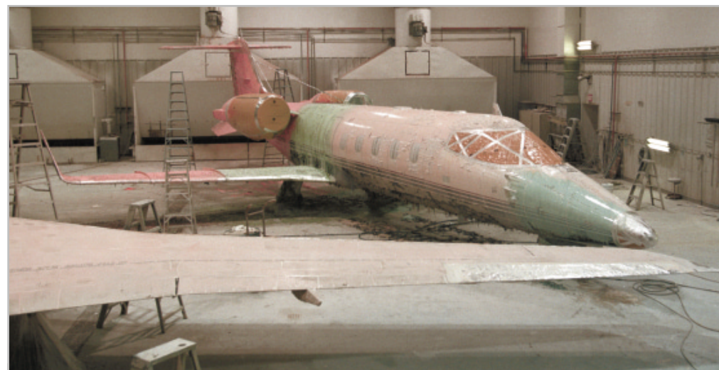
This Learjet 55 was the center of a chemical stripping experiment to find products that are safe for the environment yet provide the results the corporate aviation industry demands.
