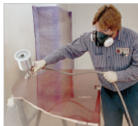
Eddie Todd, Finish Specialist, applies a high-gloss finish to an aircraft cabinet. Duncan Aviation's Finish Team applies exotic woods, finish processes and meticulous faux painting to create beautiful aircraft cabinetry.
